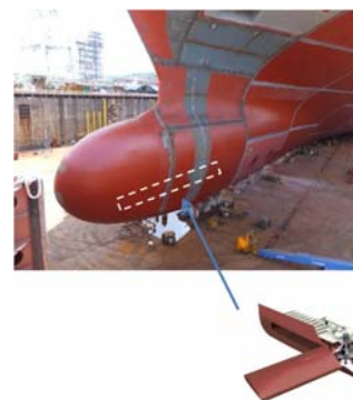
Fig. 1 Install of an extractable bow fin in a bow bulb
