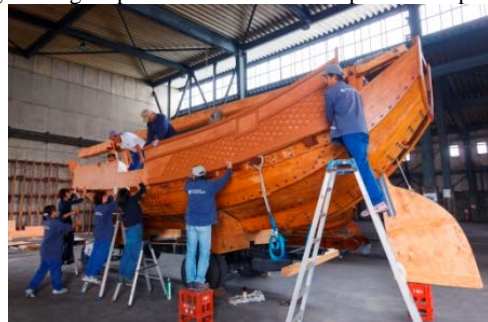
Fig.14 fabrication and setting of "Higaki Pattern"
