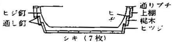
Fig. 8 The midship section of a large-sized GOHEITAFUNE
