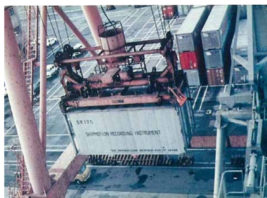
積み込み中の計測コンテナ(SR125)の文字が見える Hung-upped "measurement container" to a container ship. Letters SR125 can be seen.
