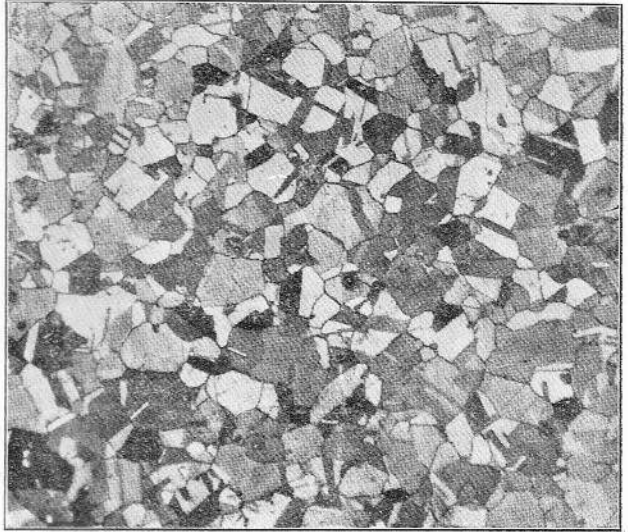
Fig. 3. Monel Metal, Cold-rolled and Fully Softened by Correct Annealing, \times 100 .
